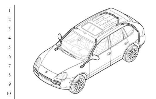
12 24. The sunroof drains lead from the roof to the wheel wells, where they are13 designed to drain water onto the ground. When the drains fail, water enters the cabin.
