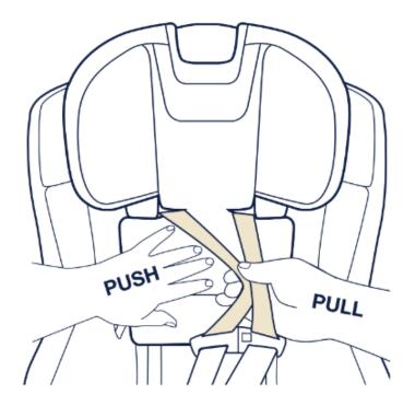
If the harness lengthens while performing the test, STOP using the seat and contact Nuna immediately.
