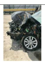
1043. On April 10, 2019, an inspector for Toyota USA inspected the wreckage of this vehicle. The EDR data recovered from the Avalon had no record of the crash. This was a sign of ASIC EOS.
