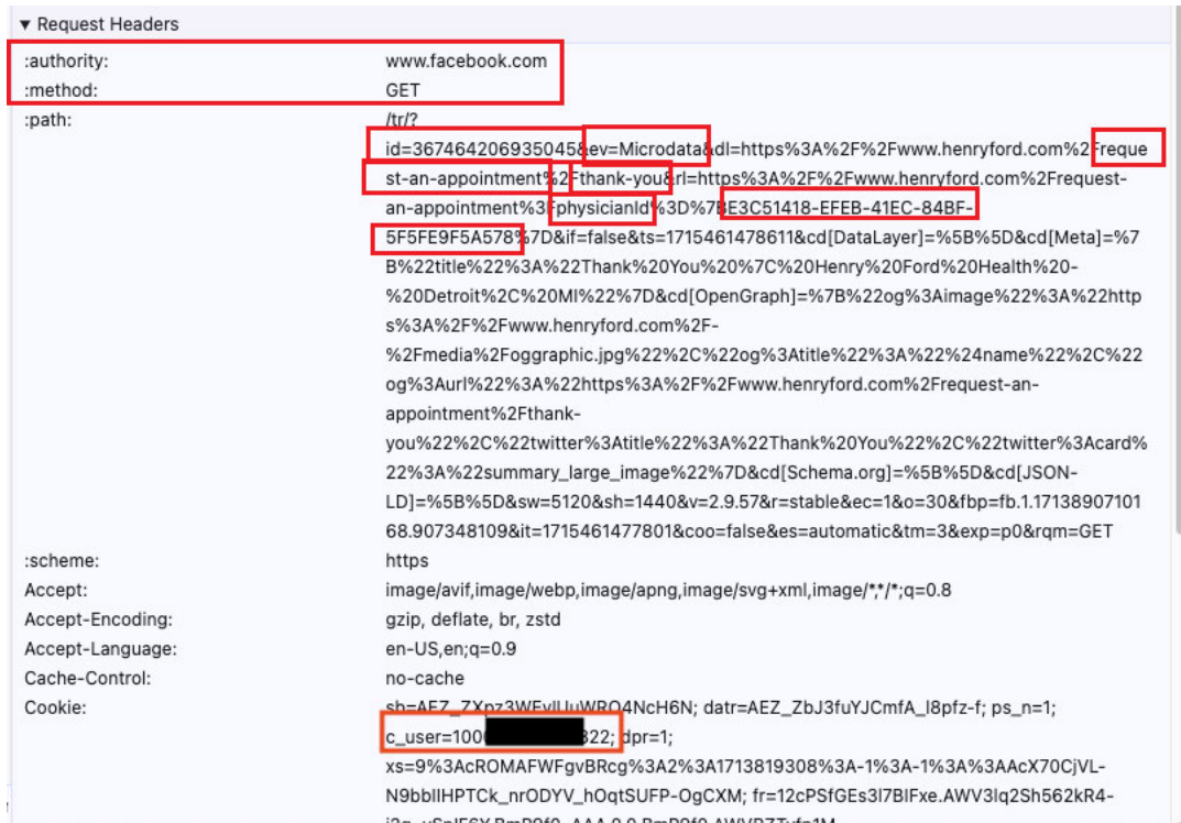
Figure 8. Screenshot demonstrating disclosure of the user’s appointment activity along with their c_user id cookie value.
