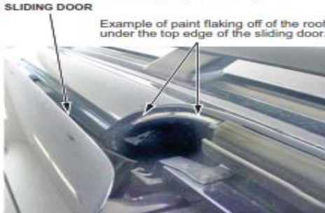
8 Example of paint flaking off the roof, under the top edge of the tailgate.
