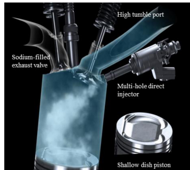
Figure 4. The components of the combustion system
