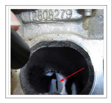
^Valves stems may have deposits build up on them. These deposits are characteristic of a direct inject engine. The valves stems do not need to be cleaned as they are not affecting engine performance (Refer to picture above).
