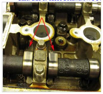
^Camshafts and roller follower will have wear markings. This is normal and do not need to be replaced (refer to picture above).
