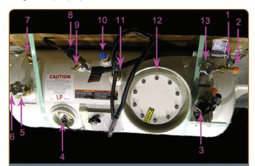
LPG Tank Components (front tank of 3-tank system shown)
