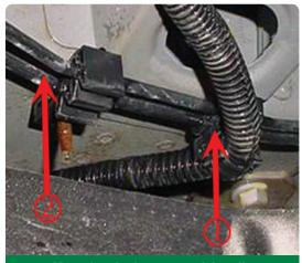
Move the wire harness retaining clip from the steel lines (1) to in front of the steel line support (2).
