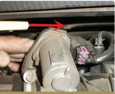
Inspect for purge pipe contact with the throttle body.
