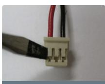
Remove the power (red +) wire from cavity #1 and the ground (black -) wire from cavity #3.
