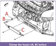
Clamp the hoses (A, B) before disconnecting the power steering cooler (C).
