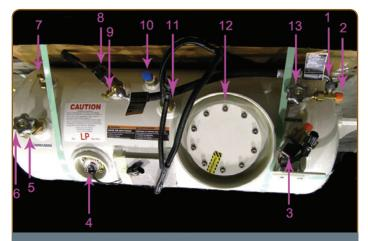
LPG Tank Components (front tank of 3-tank system shown)
