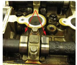
timing chain guides — that should be inspected for excessive wear as well as normal wear markings of other components, such as markings on the camshafts and roller follower.
