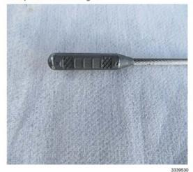
If the oil consumption test indicates that the rate of consumption is greater than 1 quart (0.946 L) of oil every 2,000 miles (3,200 km), note the oil consumption rate, the date that the ECM was reprogrammed and any
