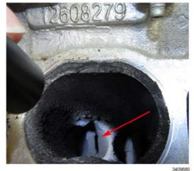
Valves stems may have deposits build up on them. These deposits are characteristic of a direct inject engine. The valves stems do not need to be cleaned as they are not affecting engine performance (Perfor to picture above).
