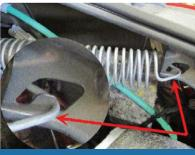
The trunk lift springs should be in the rear position.
