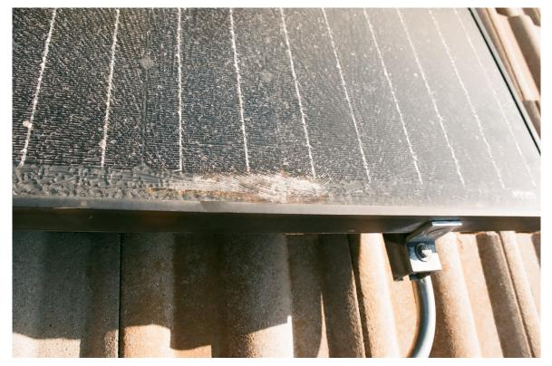
Model No. BP 4175B (Allagas Property) Burn Mark and Shattered Glass from Junction Box Failure
