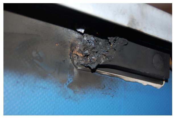
Model No. BP SX3 150S (Back) Melted junction box due to overheating caused by junction box failure.
